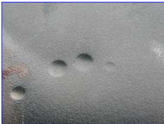
Thermolon™ Exterior - even at drop height 1,500 mm, metal substrate deforms, but the coating does not crack or delaminate
